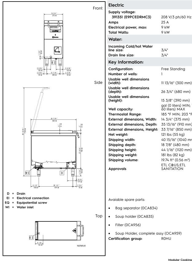
Modular Cooking Range Line Electric Freestanding Rethermalizer, 1 Well - 16gal (60 litres)
